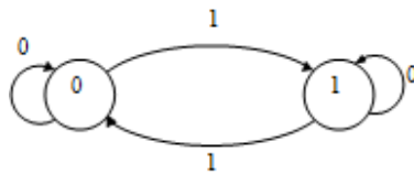
State diagram of T FF
